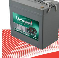
The DAB series batteries are designed to have a large amount of stored current discharged between charging sessions, with very heavy non-porous battery plates to withstand repeated major discharging and charging cycle(deep cycle). The Deep-cycle batteries uses a different chemistry for the plates active paste material, and a slightly stronger electrolyte than normal battery electrolyte, which allows for a much longer life in deep cycle applications.
